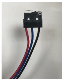
Expand the Indicator's capabilities by performing an electrical operation. Simply add the optional Micro-Switch to turn off and on motors or lights, sound a horn or alarm, etc.
